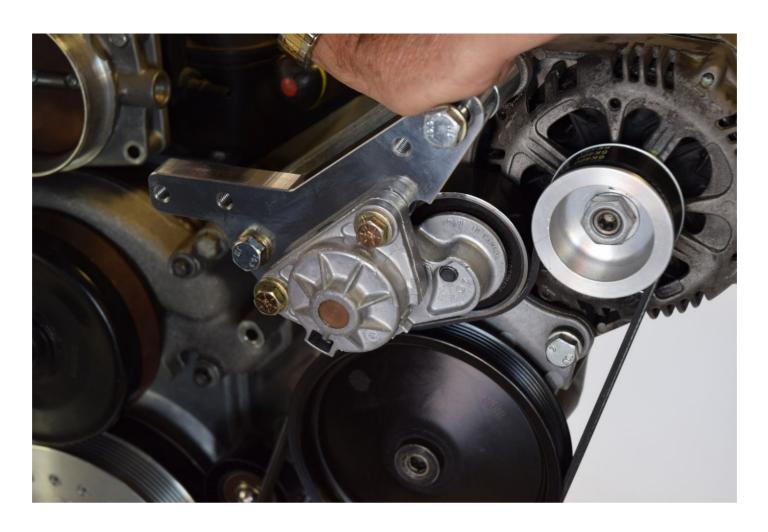
ROTATE UPPER BRACKET AND TENSIONER INTO PLACE
