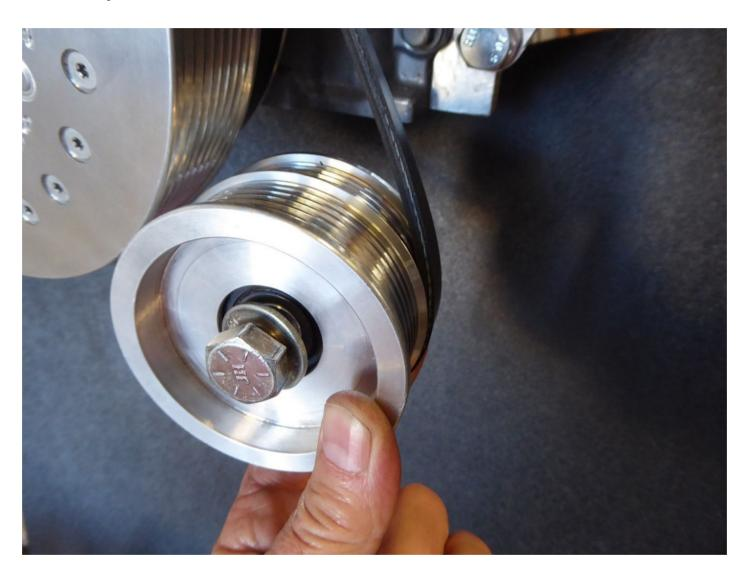
WITH PULLEY AND SPACER INSIDE THE BELT- MOVE WHOLE ASSEMBLY TO LINE UP WITH 1/2" HOLE IN THE MOUNTING PLATE
